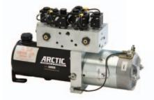
M3500V SERIES HYDRAULIC POWER UNIT The M3500V power unit has been designed around the proven M3593. The valve block has been changed to a 7 valve configuration to drive the double acting wing rams. This unit offers one of the highest power outputs in the industry, which means faster operation and less wear on the battery. Standard operating pressure is 2200 psi. Four crossover relief valves are set at 3000 psi.
